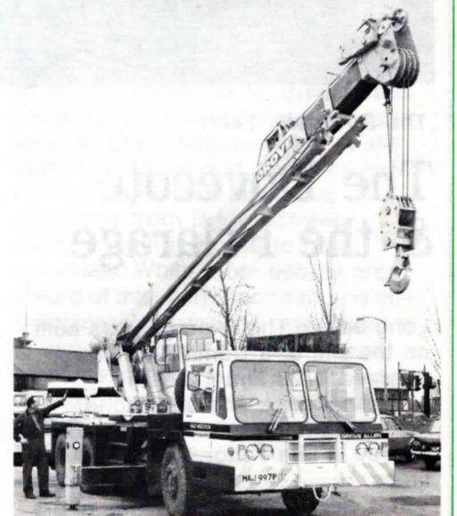
This 18 tonne capacity crane, recently acquired by HWPEL Thornaby construction department for general erection purposes, is now operating successfully at the British Steel Corporation Lackenby site.
