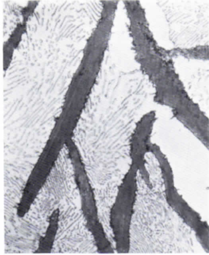
Flake graphite cast iron produced for many years at HW Iron Foundries. Magnification : \times 1000
