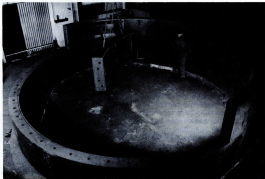
Prototype cast iron tunnel segment prior to drilling, machining and painting
