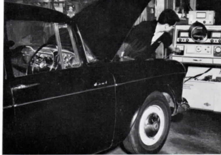
Joffre Earnshaw using modern equipment, tests the complete ignition circuit of a Humber Hawk
