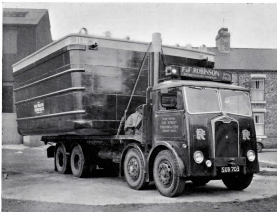
The above photograph shows a compartment boat, commonly known as "Tom Puddings," leaving the Forge Works for transport to Goole. The boat is one of a contract for fifty which has been placed with the Forge by the British Transport Waterways.
