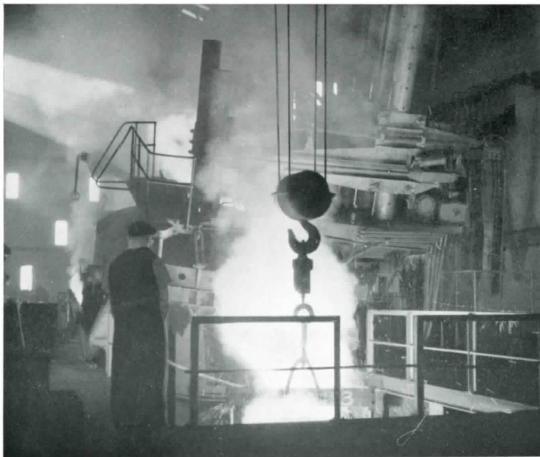
The new EFCO 10 ton 3 phase furnace in the Steel Foundry, Teesdale
